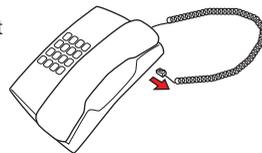
2. I) Connect the switch box cable to the telephone.
